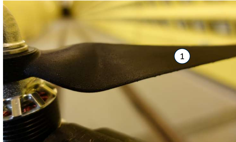
1 – formation of rain droplets on the propeller blade due to cumulus cloud simulation
