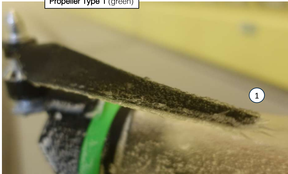
1 – after 30 sec: heavy formation of ice with long needles at the propeller tip, that break easily from time to time
